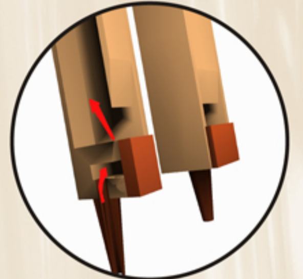
Wooden Flue Pipe
